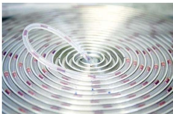
**Figure 1.** Continuous-flow spiral-shaped microphotoreactor for gas-liquid photooxygenations (LGC, Toulouse).
